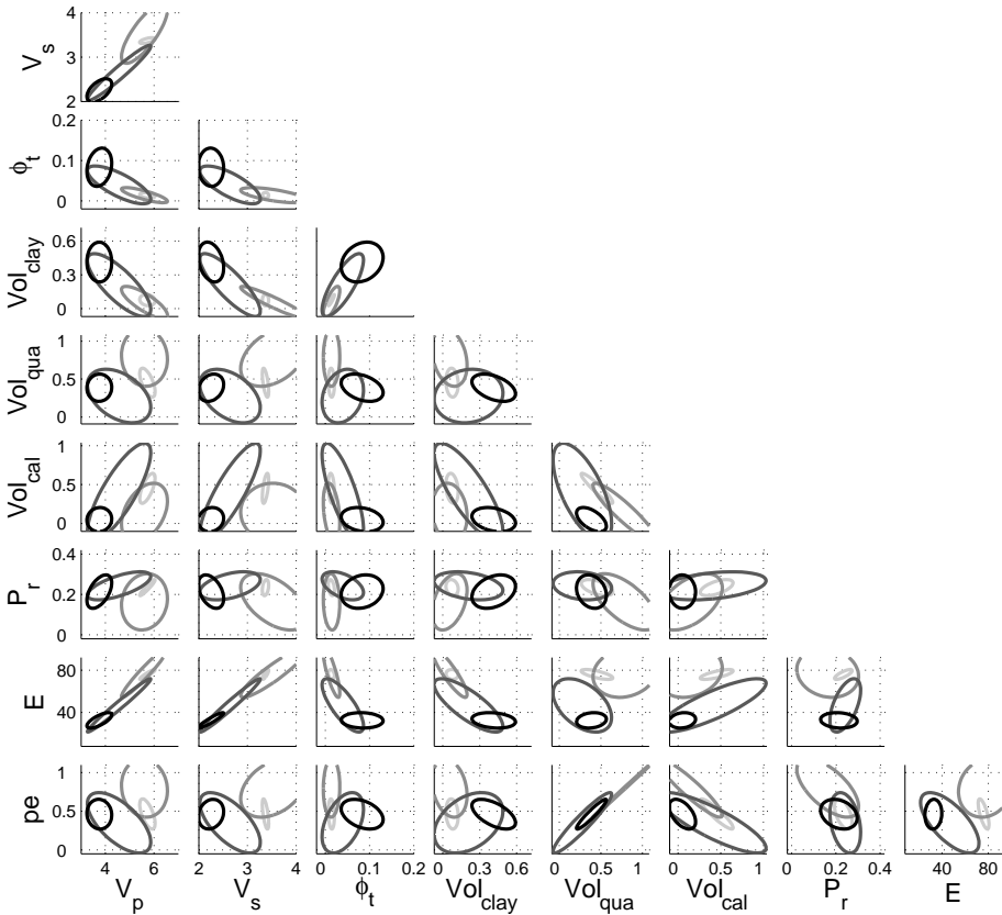
Figure 3: 2D plots of 90% confidence regions of the Gaussian likelihood model for the output probabilities for each facies class estimated empirically.
