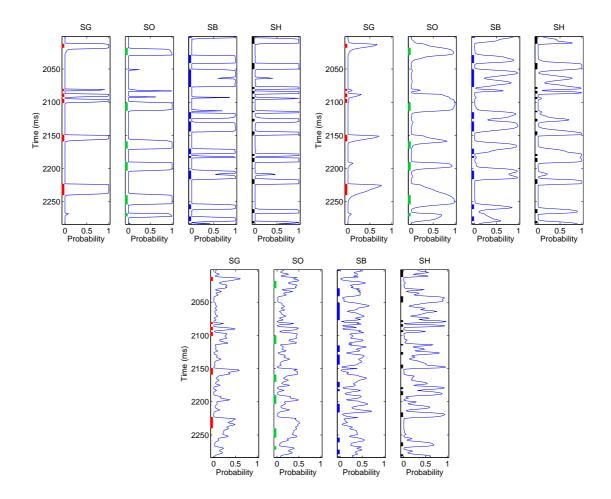
Figure 10: Marginal approximate posterior  $\tilde{p}(\pi_{\mathbf{x},t}|\mathbf{d})$  in profile  $\mathbf{x}$ : {50} for 2D Markov random field model (upper left); profilewise Markov chain model (upper right); and locationwise model (lower) with gas-saturated sandstone, oil-saturated sandstone, brine-saturated sandstone, and shale denoted SG, SO, SB, and SH, respectively. Reference LF profile  $\pi_{\mathbf{x}}$  is marked on respective axis.
