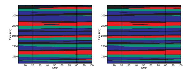
Figure 7: Locationwise most probable LF characteristics prediction  $\hat{\pi}$  for 2D Markov random field model (left); and reference LF characteristics  $\pi$  (right) with gas-saturated sandstone (red), oil-saturated sandstone (green), brine-saturated sandstone (blue), and shale (black).
