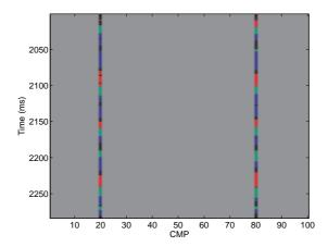
Figure 2: Well observations  $\mathbf{d}^w$  in  $\mathcal{K}$ : {20,80} with gas-saturated sandstone (red), oil-saturated sandstone (green), brine-saturated sandstone (blue), and shale (black).
