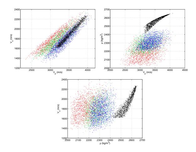
Figure 3: Elastic properties  $\mathbf{m}$  represented by P-wave velocity  $(V_p)$ , S-wave velocity  $(V_s)$ , and density  $(\rho)$  given gas-saturated sandstone (red), oil-saturated sandstone (green), brine-saturated sandstone (blue), and shale (black) simulated from a rock physics model.
