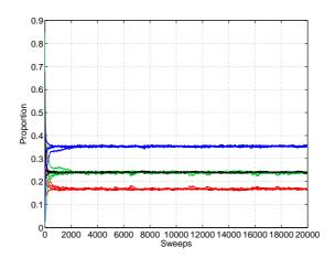
Figure 5: Convergence plot monitoring proportion of LF classes after each sweep of simulation algorithm with gas-saturated sandstone (red), oil-saturated sandstone (green), brine-saturated sandstone (blue), and shale (black).
