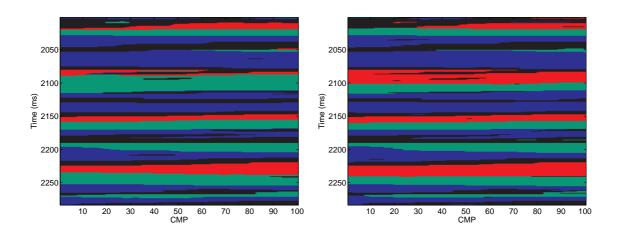
Figure 12: Locationwise most probable LF characteristics prediction  $\hat{\pi}$  for 2D Markov random field model from inversion without well observations (left); and reference LF characteristics  $\pi$  (right) with gas-saturated sandstone (red), oil-saturated sandstone (green), brine-saturated sandstone (blue), and shale (black).
