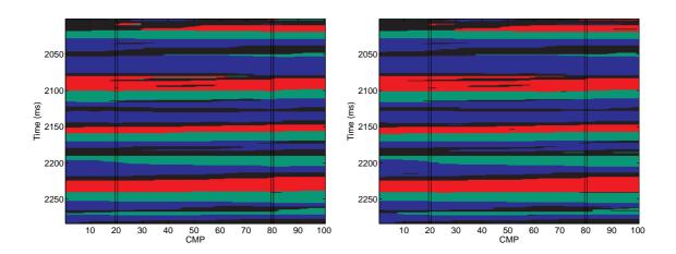
Figure 11: Results from case without observation error, i.e., inversion based on reference seismic signal s. Locationwise most probable LF characteristics prediction  $\hat{\pi}$  for 2D Markov random field model (left); and reference LF characteristics  $\pi$  (right) with gas-saturated sandstone (red), oil-saturated sandstone (green), brine-saturated sandstone (blue), and shale (black).
