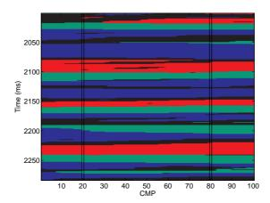
Figure 1: Reference LF characteristics  $\pi$  with gas-saturated sandstone (red), oil-saturated sandstone (green), brine-saturated sandstone (blue), and shale (black).
