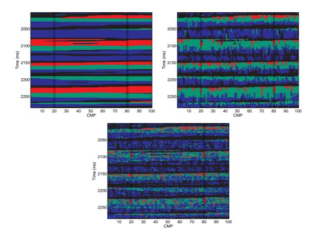
Figure 9: Locationwise most probable LF characteristics predictions  $\hat{\pi}$  for 2D Markov random field model (upper left); profilewise Markov chain model (upper right); and locationwise model (lower) with gas-saturated sandstone (red), oil-saturated sandstone (green), brine-saturated sandstone (blue), and shale (black).
