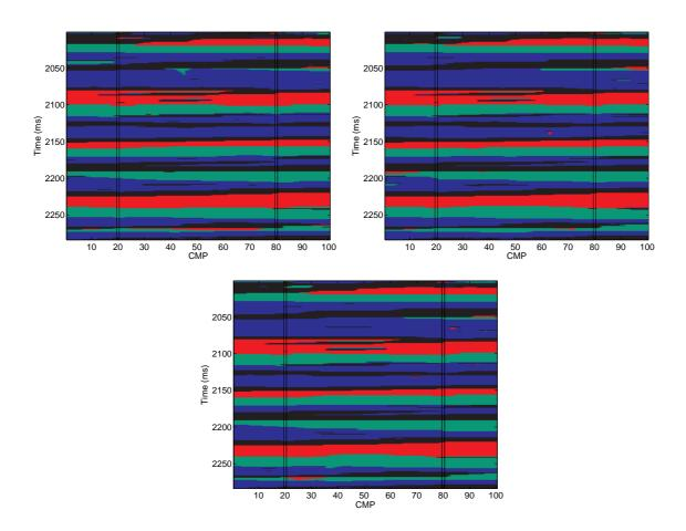
Figure 6: Independent realizations of LF characteristics from approximate posterior  $\tilde{p}(\boldsymbol{\pi}|\mathbf{d})$  for 2D Markov random field model with gas-saturated sandstone (red), oil-saturated sandstone (green), brine-saturated sandstone (blue), and shale (black).
