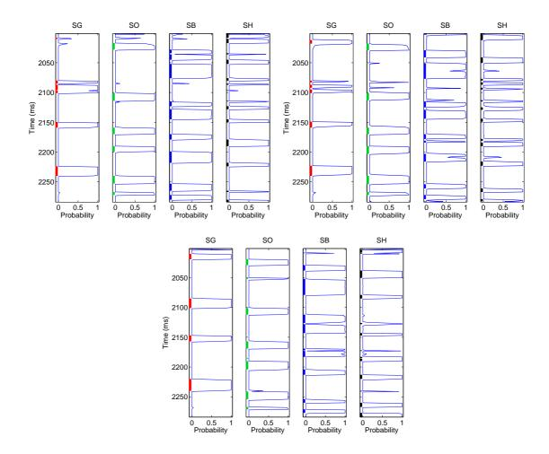
Figure 8: Marginal approximate posterior  $\tilde{p}(\pi_{\mathbf{x},t}|\mathbf{d})$  for 2D Markov random field model in profiles  $\mathbf{x}:\{21,50,79\}$  upper left, upper right and lower, respectively, with gas-saturated sandstone, oil-saturated sandstone, brine-saturated sandstone, and shale denoted SG, SO, SB, and SH, respectively. Reference LF profile  $\pi_{\mathbf{x}}$  is marked on respective axis.
