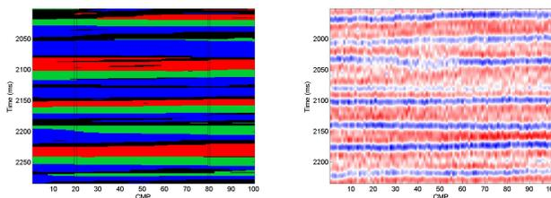
Figure 1: Reference LF characteristics  $\pi$  with two well profiles marked, with gas-saturated sandstone (red), oil-saturated sandstone (green), brine-saturated sandstone (blue) and shale (black); and synthetic seismic data  $d$  stacked from the angles  $\theta = (0, 10, 20, 30, 40)^\circ$ .
