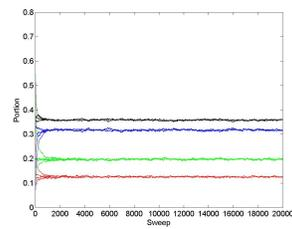
Figure 3: Convergence plot monitoring the portion of the LF classes after each sweep of the simulation algorithm with gas-saturated sandstone (red), oil-saturated sandstone (green), brine-saturated sandstone (blue) and shale (black)
