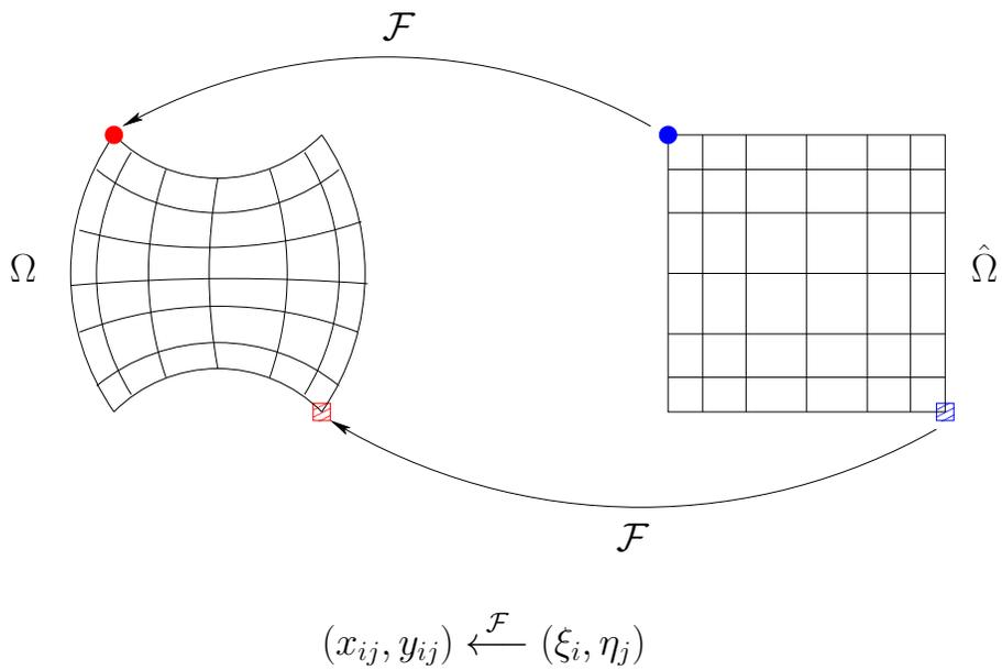
Figure 3: Each point in the reference domain is mapped to a unique point in the physical domain. In particular, the boundary of  $\partial\hat{\Omega}$  is mapped to  $\partial\Omega$ .
