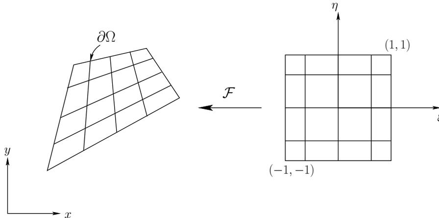
Figure 4: Each edge of the physical domain  $\Omega$  is here a straight line.
