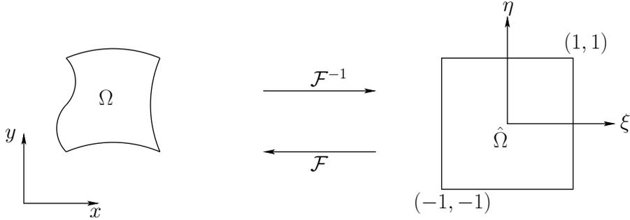
Figure 1: The two-dimensional deformed domain  $\Omega$  is here considered to be the image of the reference domain  $\hat{\Omega}$  through a regular one-to-one mapping,  $\mathcal{F}$ .
