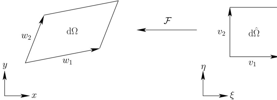
Figure 2: The surface element  $d\hat{\Omega}$  in  $\hat{\Omega}$  is related to a corresponding surface element  $d\Omega$  in  $\Omega$  via the mapping  $\mathcal{F}$ .
