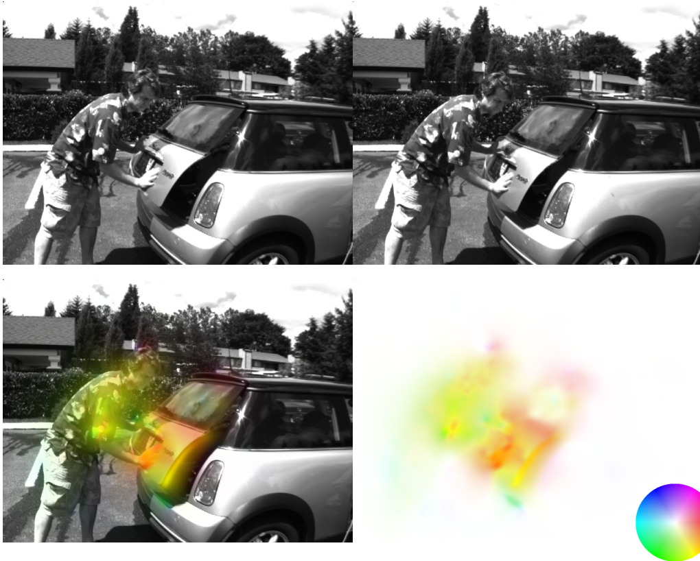
Figure 1: Result of an optical flow computation. First row: Two consecutive frames in an image sequence. Second row: The resulting flow ( right ) and the first frame of the sequence overlaid with the flow ( left ). The colourwheel on the bottom right indicates the direction and intensity of the flow field at each pixel. The test images have been taken from http://vision.middlebury.edu/flow/ . The optical flow has been computed with a regularisation parameter of \lambda = 1000 , and the images were pre-smoothed using a Gaussian kernel with standard deviation \sigma = 5 .
