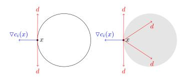
Left: Equality constraint  $c_i(x) = 0$ . Right: Inequality constraint  $c_i(x) \ge 0$ .
