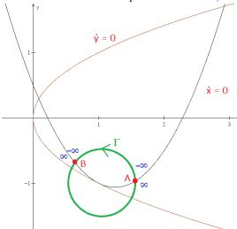
At point A, along the green curve  $\Gamma$ ,  $\dot{y}/\dot{x}$  changes from  $\infty$  to  $-\infty$ , and at point B, along  $\Gamma$ ,  $\dot{y}/\dot{x}$  changes from  $-\infty$  to  $\infty$ . These are the only points along  $\Gamma$  at which  $\dot{x}=0$  and  $\dot{y}\neq 0$ , and hence the only points at which  $|\dot{y}/\dot{x}|=\infty$ .
