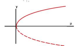
The red lines indicate the locations of the fixed points as  $\mu$  varies away from 0. The dashed line indicates an unstable fixed point and a solid line indicates a stable fixed point. We call this type of bifurcation a SADDLE-NODE BIFURCATION. The statement that these transversality conditions guarantee a saddle-node bifurcation is known as Sotomayor's Theorem (see *Perko*, pg. 338).
