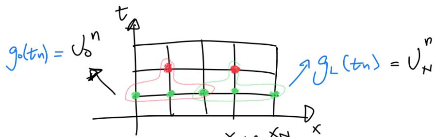
$$\rightarrow i=N-1 : \overset{\circ}{U_{N-1}^{n+1}} = \alpha \overset{\circ}{U_{N-2}^n} + (1-2\alpha) \overset{\circ}{U_{N-1}^n} + \alpha \overset{\circ}{U_N^n}$$
