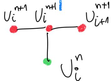
$$\frac{\partial u}{\partial t} = c^2 \frac{\partial^2 u}{\partial x^2} \Rightarrow \frac{U_i^{n+1} - U_i^n}{\Delta t} = c^2 \left( \frac{U_{i+1}^{n+1} - 2U_i^{n+1} + U_{i-1}^{n+1}}{\Delta x^2} \right)$$
