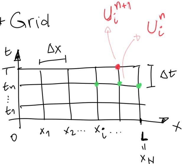
Forward:  $\frac{U_i^{n+1} - U_i^n}{\Delta t} = c^2 \left( \frac{U_{i+1}^n - 2U_i^n + U_{i-1}^n}{\Delta x^2} \right)$
