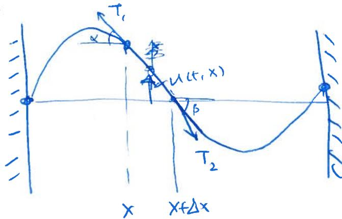
$$\begin{aligned} T_1 \cos(\alpha) &= T_2 \cos(\beta) \\ &=: T \end{aligned}$$
