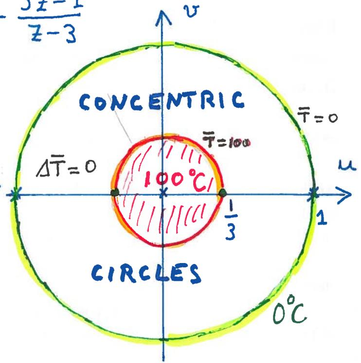
$$\frac{\partial^2 T}{\partial x^2} + \frac{\partial^2 T}{\partial y^2} = 0 \iff \frac{\partial^2 \bar{T}}{\partial u^2} + \frac{\partial^2 \bar{T}}{\partial v^2} = 0$$
