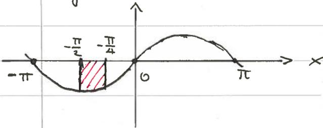
$$\begin{aligned} A &= \int_{-\pi/2}^{-\pi/4} \sin x dx \\ &= [\cos x]_{-\pi/2}^{-\pi/4} \\ &= \cos\left(-\frac{\pi}{4}\right) - \cos\left(-\frac{\pi}{2}\right) = \frac{1}{\sqrt{2}} \end{aligned}$$
